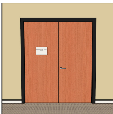
Sign on inactive leaf at double-door entry
