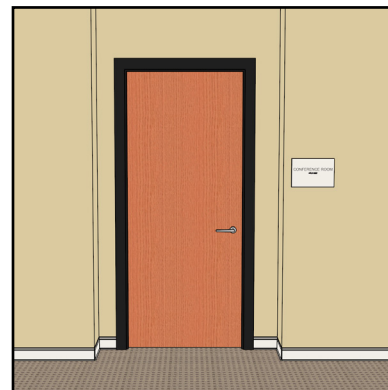
Recessed door with sign on adjacent wall
