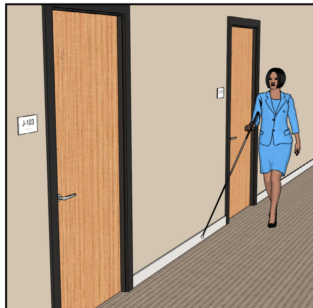
Doorways provide a tactile cue for locating signs.
