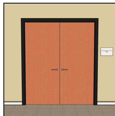
Sign at right-side hinge side of double-door entry with two active leaves
