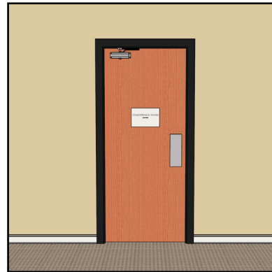
Sign on push side of a door with a closer
