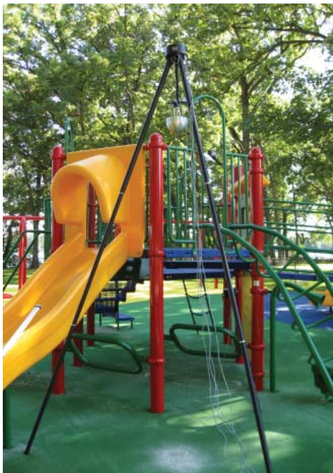
A TRIAX is used here to test impact attenuation or the play surface’s ability to absorb a fall and reduce severity of injury.
